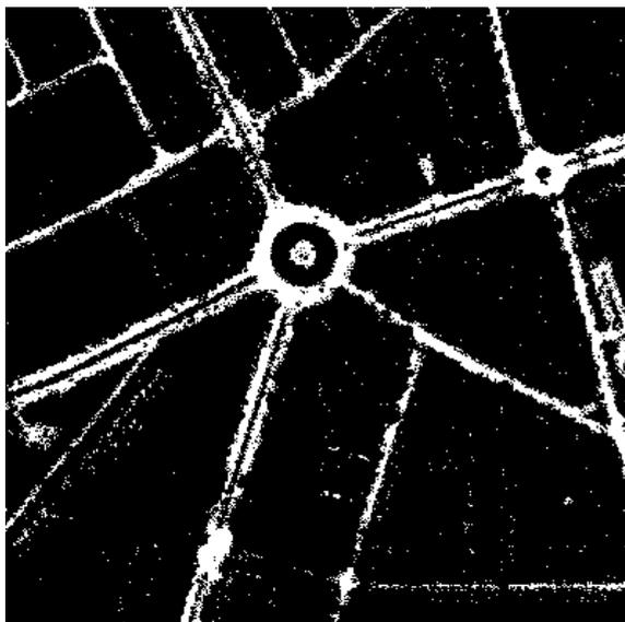
*Figure 7. Road detection using SVM classifier.*
