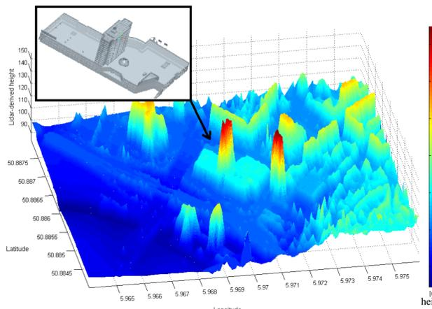
Fig5. Lidar-derived (AHN-1) height map over the area, interpolated from 5 to 0.5 m resolution. Shopping mall 't Loon' (3D model inset) is indicated by the black arrow. Note that the high-rise apartment of 't Loon' is smoothed by the interpolation.
