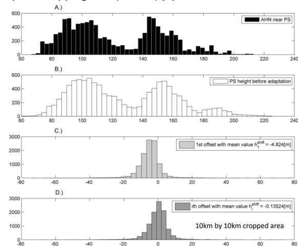
Fig7. A.) Height distribution of Lidar points closest to PS points (<5m). B.) Original distribution of PS height. C.) height difference distribution between Lidar and PS, yielding an initial offset value of -4.824m. This yields new horizontal positions of the PS. D.) Final offset after the iterative estimation. The iteration will continue until the offset value is below AHN vertical resolution (15cm).
