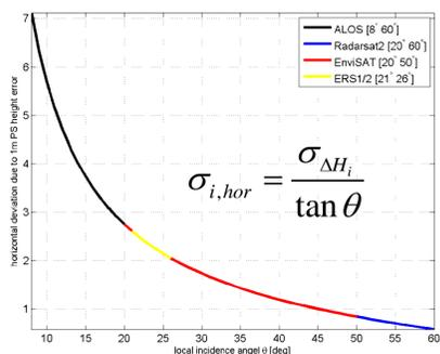
Fig2. Horizontal deviation due to PS height estimation error of 1m for ALOS, Radarsat-2, Envisat and ERS-1/2. For most sensors the horizontal shift is 1.5-3 times the vertical error.
