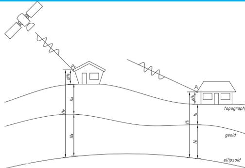
Fig1. Relationships between reference surfaces: topography, geoid and ellipsoid with two points  $P_0, P_i$ .
