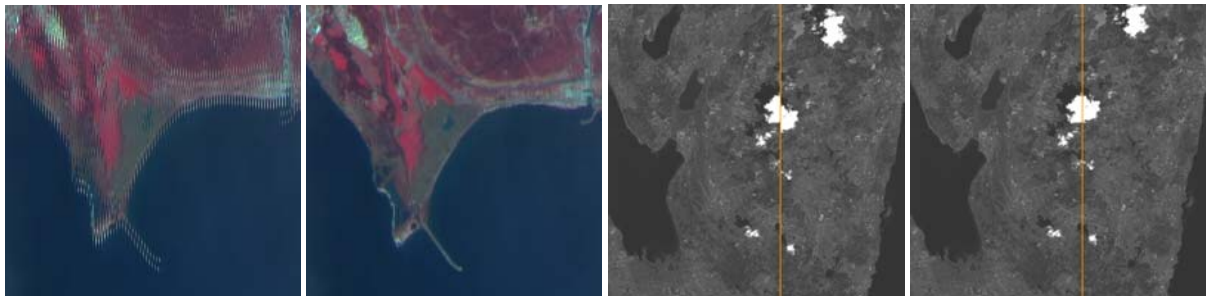
Figure 1. ALOS and EnMAP co-registration (1 st and 2 nd : AVNIR-2 real mission data, 3 rd and 4 th : EnMAP simulated mission data; 1 st and 3 rd : not co-registered, 2 nd and 4 th : co-registered)
