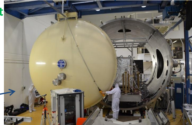
MSI PFM during thermal test (AirbusDS-F & CSL-B)
