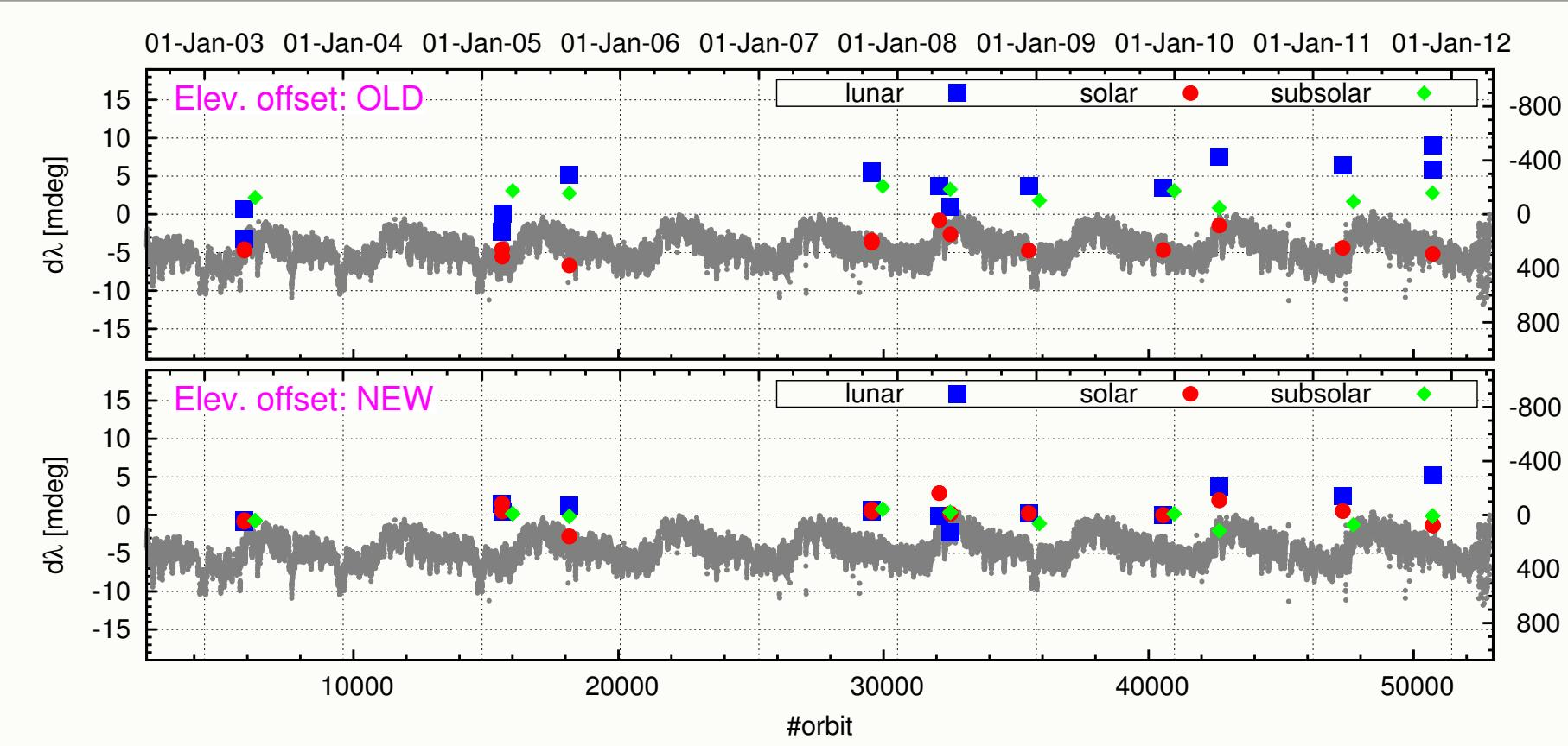
► Elevation angle offset (EAO) minimized for all measurement types.
