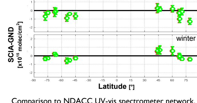
Comparison to NDACC UV-vis spectrometer network.
