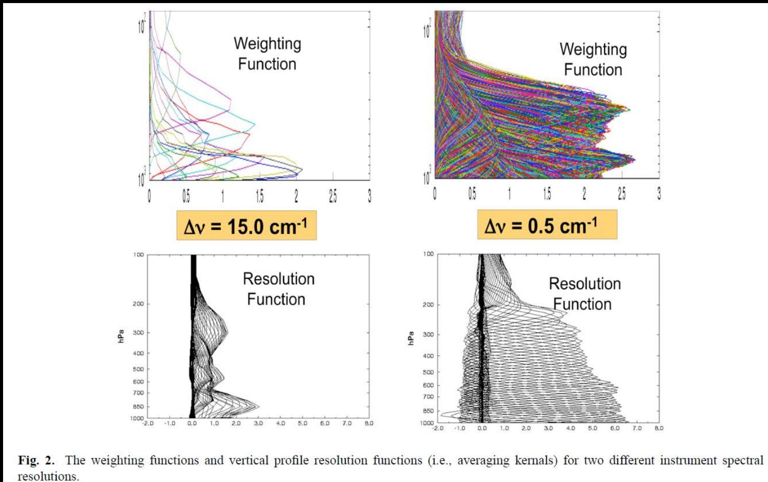
**Fig. 2.** The weighting functions and vertical profile resolution functions (i.e., averaging kernels) for two different instrument spectral resolutions.
