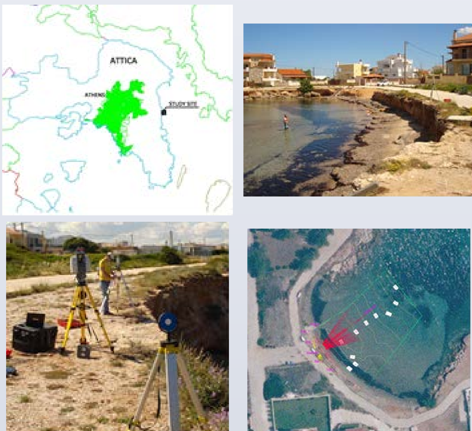
Figure 1. a) The study site b) The deployment of the TLS (Terrestrial Laser Scanner), the TS (Total Station) and one of the spherical targets in the field site c) Measuring bathymetry by classical surveying techniques. Orthophoto of the beach field site with over-imposed bathymetric contours derived from Total station bathymetric survey and with the TLS position and scanned area.
