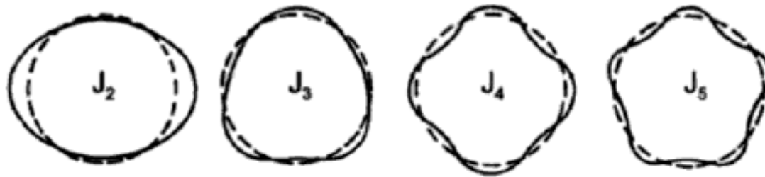
Figure 2.2: Illustration of the oscillation of the Legendre functions in the latitudinal direction, also known as the zonal harmonics. Notice that the Legendre polynomials only exist on the interval \theta \in [0; \pi] , meaning that these figures should be viewed as a cross-section of the Legendre polynomial, rotated around the north-south axis. The figure is from Messerschmid and Bertrand (1999)
